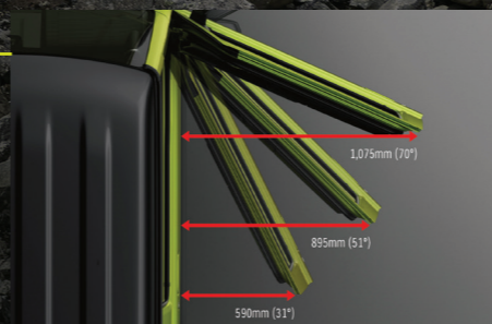
FRONT DOOR OPENING
